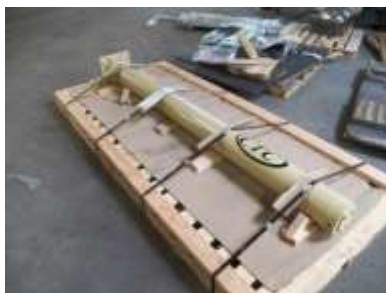
★ WELDED TRAMPER CYLINDER 6" X 4" X 78" TVL RATED @ 3000 PSI
