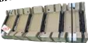
6 TIE UPPER PLATEN WITH TIE BARS
