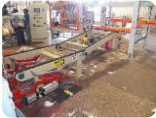
BALE LIFT CONVEYOR TO FIT THE FISHBURNE PRESS & LP BROWN BAGGER
