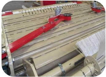
ROTARY SLITTER KNIFE & KNIFE ARM
