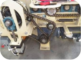
DRIVE SYSTEM FOR SPIKE, SHELL, & FEED ROLLERS W/O COVERS
