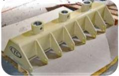
• Dimensionally interchangeable except for height which is 1 ½" more than original. This allows tramper foot to extend further below the dogs eliminating the need to purchase a longer stroke tramper cylinder.
