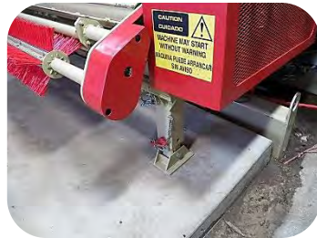
ADJUSTABLE JACK LEG & SWEEPER DRIVE
