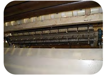
DOFFING SYSTEM AS VIEWED FROM BELOW
